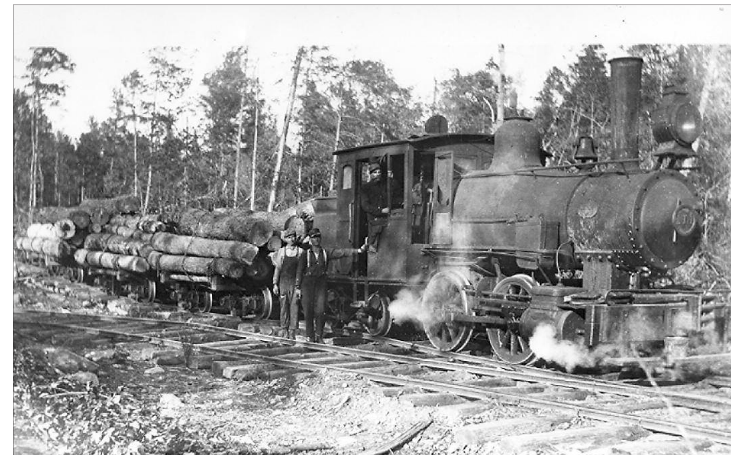
▲ The former LSE #15 at the lumber operation of John S. Dalton in the Chase - Big Rapids area of west central Michigan about 1902-3. It is seen here with a distinctive headlight platform, oil-burning headlight, and new number plate. The rear sandboxes have been removed leaving one per side, with a very large box above the running board to increase its capacity. It is only equipped for link and pin couplings. The truck wheels have been changed from the original spoked type to solid wheels. The circular item on its roof is a remnant of the cab top marker lamps and discs used on the elevated. It is now a simple locomotive with a cover over the former receiver opening under the builder's plate. —Bentley Historical Library, University of Michigan
